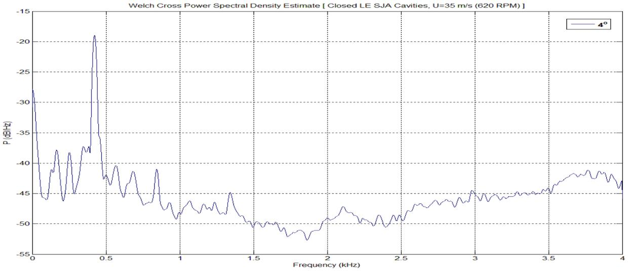
**Figure 12:** Pressure Spectra at 4 deg AoA, Slots Closed
