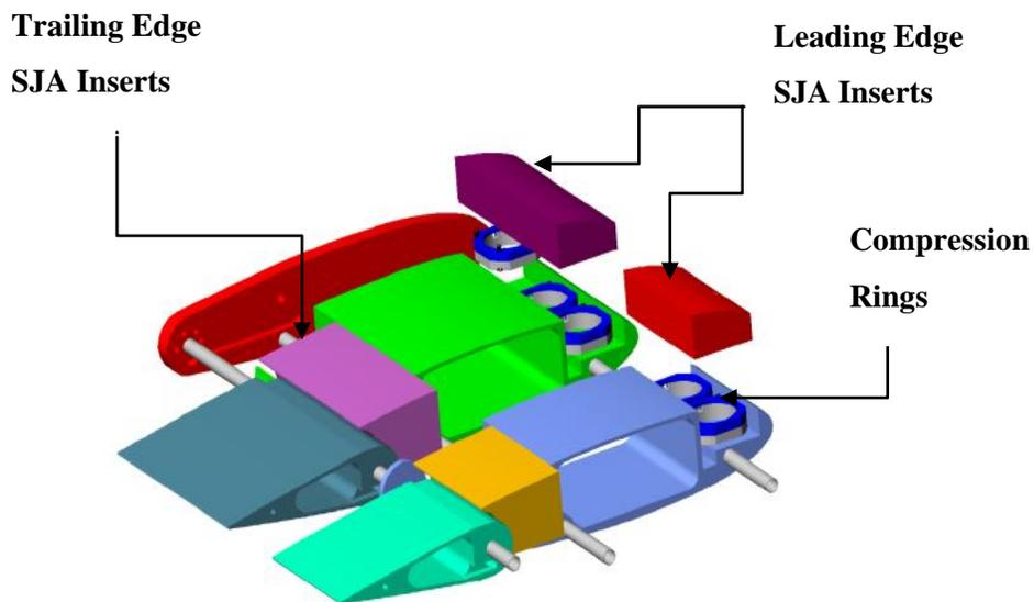
**Figure 2:** Partial Wing Assembly
