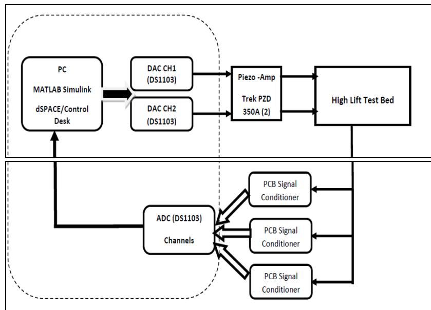
**Figure 5** Schematic of experimental setup
