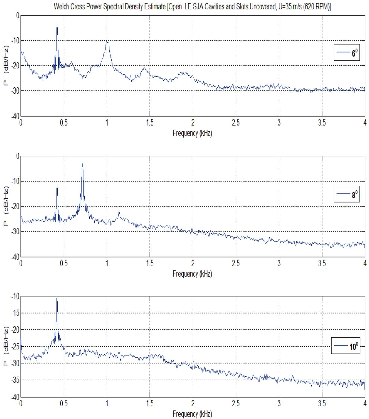
**Figure 9:** Pressure Spectra for AoA=6-10 degs
